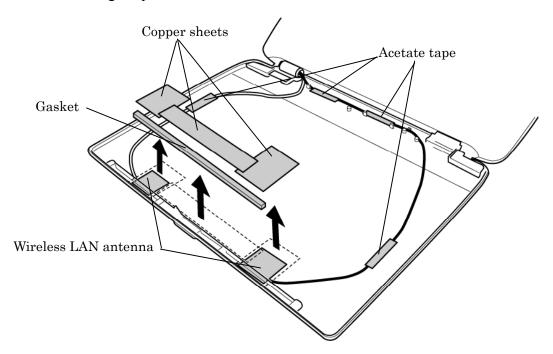
Figure 4-45 Removing the wireless LAN antenna
